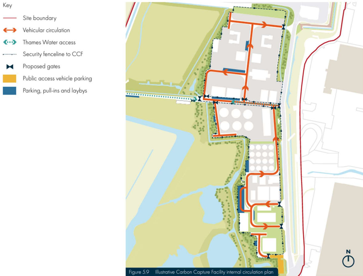
Figure 8- Carbon Capture Facility Circulation Plan
